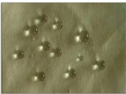
Figure 4. Water droplets on super hydrophobic titania hybrid coated a) fabric b) paper.
